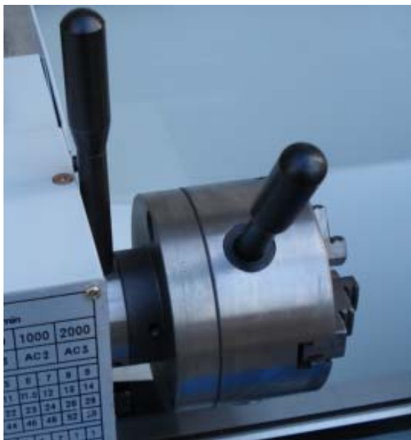
Figure 2 . Chuck removal bars in place
